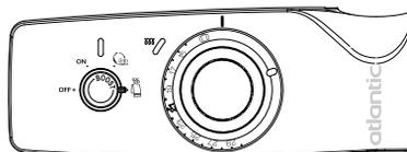
Another example : The wheel **D** is set to 21°C. The temperature displayed on your thermometer is 18°C. The calibration value will therefore be -3°C (3 notches).
