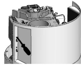
⑥ Loosen the cable clamp on the rear cover to pass the optional equipment cable (not supplied) through it.
