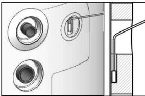
**3** Insert the sensor in the neck, ensuring that it is correctly positioned at the bottom of the housing.
