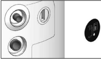
**1** Remove the magnet from the housing next to the internal heat exchanger branch connections...
