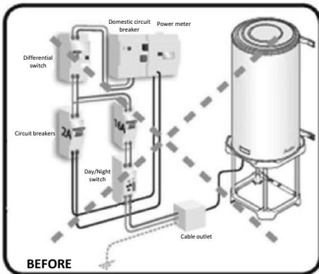
Installing the hot water heat pump
