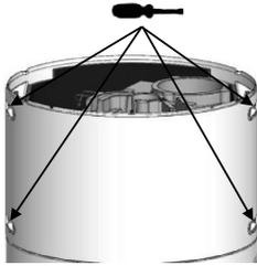
④ Remove the covers and unscrew the 4 screws on the front cover of the heat pump.
