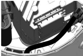
⑦ Route the cable through the passage specifically designed for access to the PCB.
