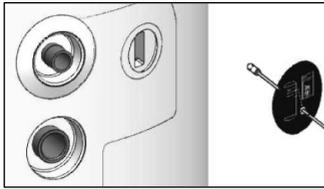
**2** Pass the temperature sensor through the magnet (the magnet has been drilled for this purpose).
